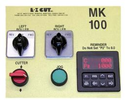
Way Cutter, you can make your next cut by pushing & holding the Cutter Switch to REV. Your Cutting Bar's Cable may require periodic lubrication. If the Cutter makes a vibrating (humming) sound when running, lightly lubricate the Cutting Bar Cable with a water-based lubricant such as WD-40. Spray the Cable at the top of the middle pulley just under the Cutting Track. Run the Cutter back and forth a few times to work the lubricant in and then wipe off any excess.
